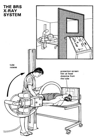
Fig. 1-8 THE BRS X-RAY SYSTEM was developed by WHO to make essential cost-effective radiology available safely and reliably all over the world. If you want one of these machines, order one made to WHO specifications. Note the screen protecting the operator. *Kindly contributed by Philip Palmer.*
