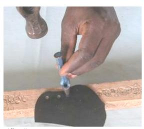
Then cut out using a pair of scissors (fig 4). Punch 6 mm holes for the shoelace (fig 5).
