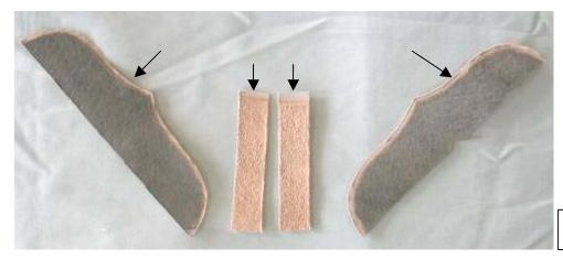
Roughen the outside part of the leather if "thin leather" was used. This will later be glued on the inside of the upper leather (fig 7).
