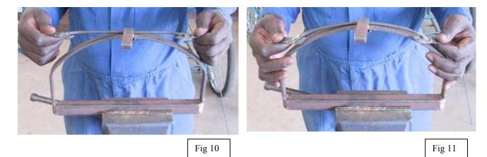
Note: when the child has a clubfoot only on one side, the abduction bar should be bend to the normal 30-40 degrees external rotation for the normal foot.
