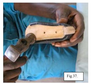
TIP: Shape the end of a piece of timber in such a way that it fits in the shoe, especially in the heel. Let this piece of timber rest on the floor and put the brace over it. Hammer gently. It will now work as a triple iron/pronge (fig 37).
