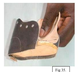
Apply glue on the outside edge of the outersole and on the leather that was left over as lasting allowance. Let it dry and connect both parts by folding the leather onto the plywood. Hammer gently to get good bonding (see fig. 36 & 37).
