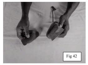
Apply glue again on the sock lining and on the cardboard insole inside the shoe. Let it dry. Attach firmly (see fig 42 & 43).
